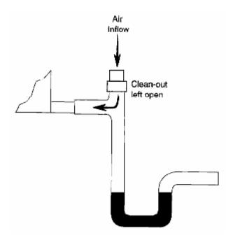
Due to this inherent maintenance concern, many traps are equipped with clean-out openings as indicated in <u>Figure 4</u>. One common problem is that these drain "clean-outs" are left open to facilitate easier access in the future. When open, untreated air can flow directly into the system causing the same problems as no trap at all.
