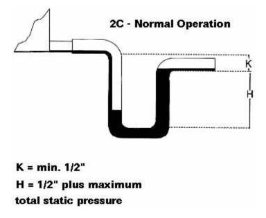
Figure 2 shows the relevant dimensions for a properly constructed positive pressure trap.
