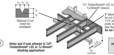
8" diameter max. hole may be cut in blocking panel for 11%" ioists: 6" max. for 91/2" joists or blocking panels less than 12" long. Do not cut flanges.
