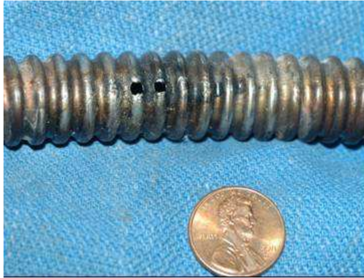
Figure 10: Adjacent perforations in CSST
