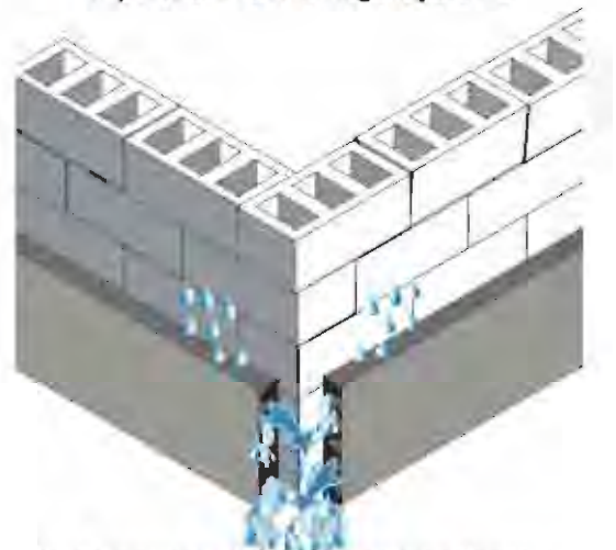
How the Geocomposite Soil Drainage System works
