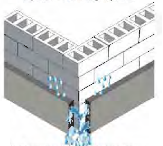
How the Geocomposite Soil Drainage System works
