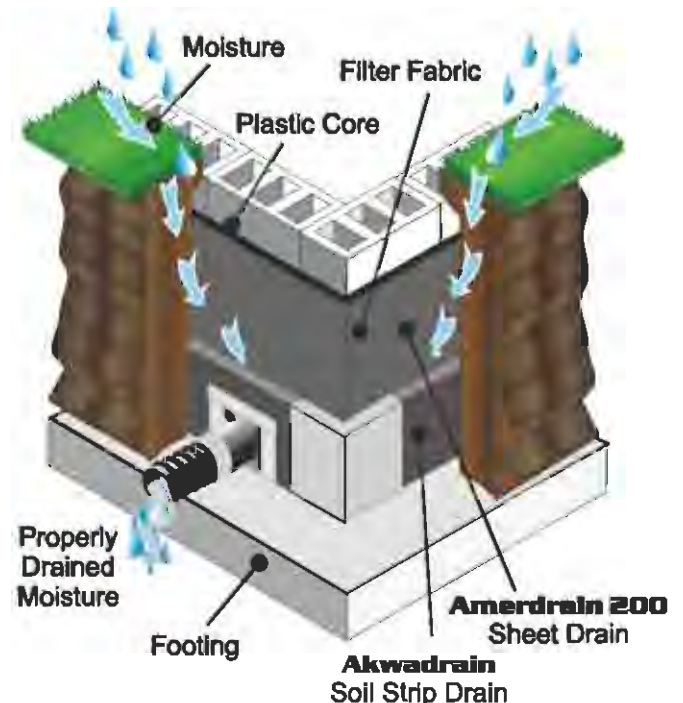
How the Geocomposite Soil Drainage System works
