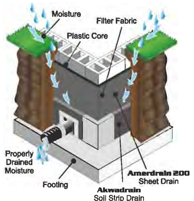
How the Geocomposite Soil Drainage System works
